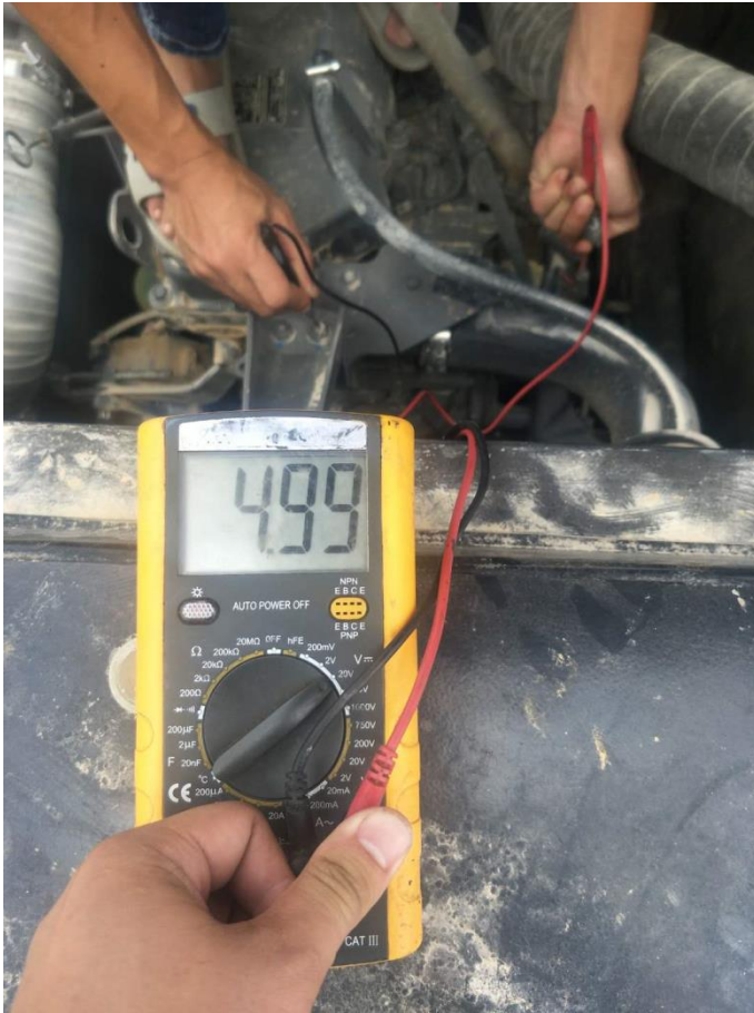
拔下传感器插头，5V及接地正常
